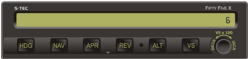
Fig. 2-2. AP Display, Software Revision Number
