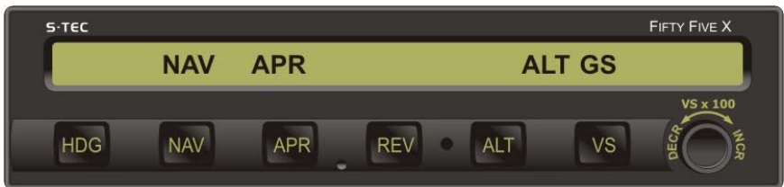
Fig. 3-18. AP Display, NAV APR and ALT HOLD Modes Engaged, GS Mode Armed
