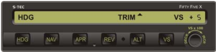
a. TRIM UP in Progress
