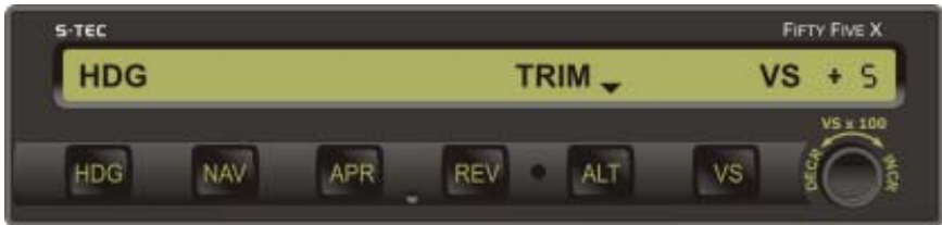
b. TRIM DN in Progress
