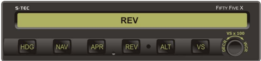
Fig. 3-34. AP Display, REV Mode Engaged, Track VOR Front Course Outbound
