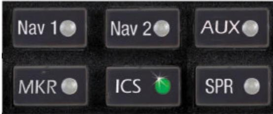
If the aircraft is equipped with a DME or ADF, these audio sources can be selected with the AUX button.
