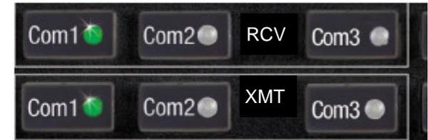
speaker (if selected). You can check this function by switching from COM 1 to COM 2 and watch the selected audio light on the selector change from COM 1 to COM 2. This ensures the pilot will *always* hear the audio from the transceiver he is transmitting on.
