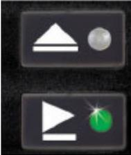
The top button is used to stop and eject the disc. Press momentarily to stop, press and hold to eject. Pushing BOTH buttons momentarily will cause the CD to “back up.” If pushed in mid song, it will back up to the beginning of the track. At the beginning of a song, it will go back to the previous track.
