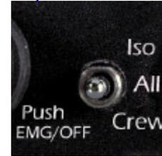
**ISO: (Up Position):** The pilot is isolated from the intercom and is connected only to the aircraft radio system. He will hear the aircraft radio reception (and sidetone during radio transmissions). Copilot will hear passengers' intercom and Entertainment 1, while passengers will hear copilot intercom and Entertainment 2. Neither will hear aircraft radio
