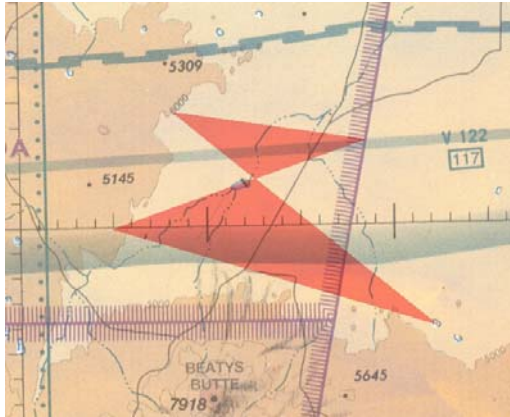
FIGURE 6-12 Bow-Tie TFR Resulting From Coordinates Out of Sequence
