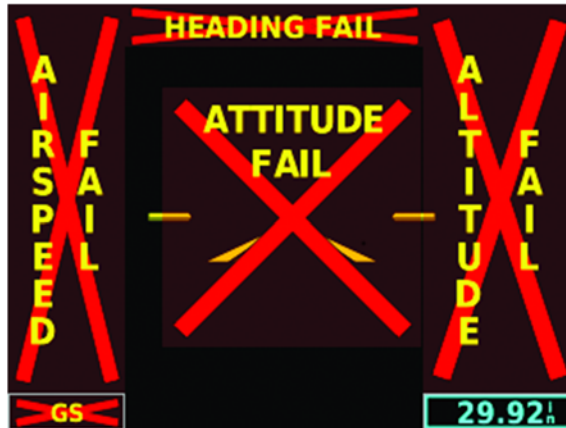
G5 ADI Failure Indications
