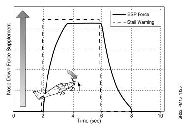
Engagement Limit:.....Stall warning Maximum Stick Force attained at:..... 1.5 seconds after stall warning Disengagement Threshold:......Stall warning deactivated Zero Stick Force: ......2 seconds after stall warning deactivated
