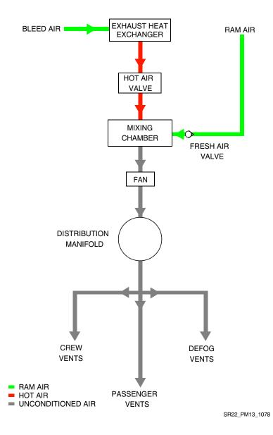
Figure 13-2: Air Conditioning System (if installed)
