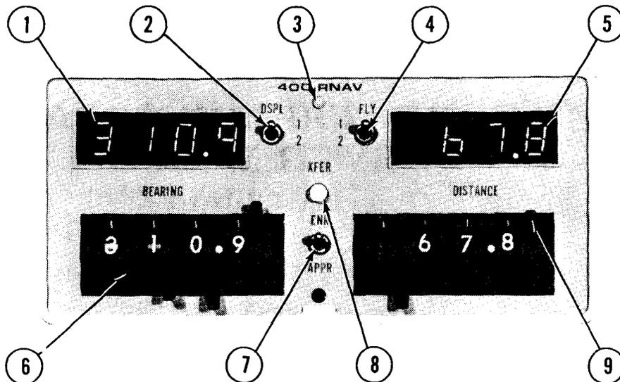
1. BEARING DISPLAY READOUT - Depending on position of DSPL Switch, displays bearing programmed for waypoint 1 or waypoint 2.
