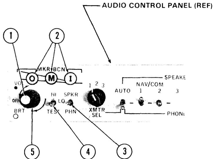
1. OFF/VOLUME CONTROL (OFF/VOL) - The small, inner control turns the set on or off and adjusts the audio listening level. Clockwise rotation turns the set on and increases the audio level.
