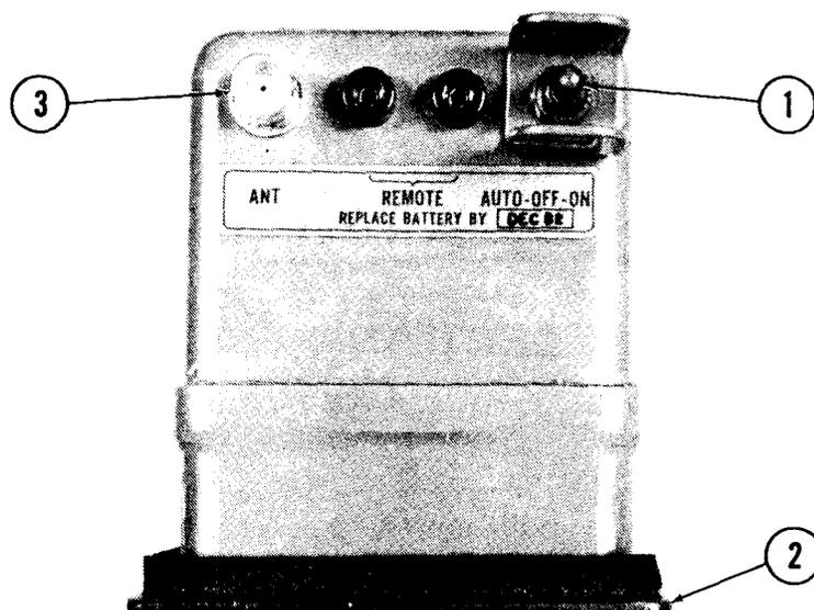
1. FUNCTION SELECTOR SWITCH (3-position toggle switch):
