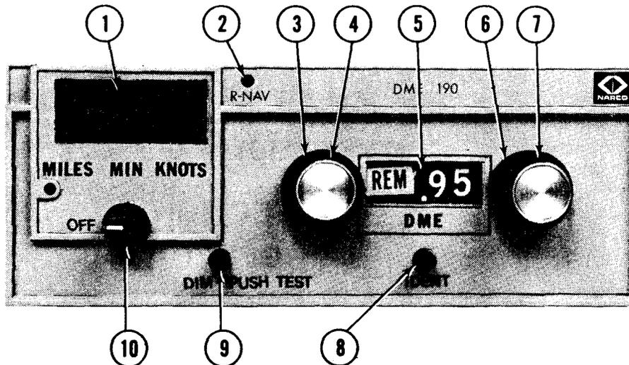
1. READOUT WINDOW - Displays function readout in nautical miles (distance-to-station), minutes (time-to-station) or knots (ground speed).
