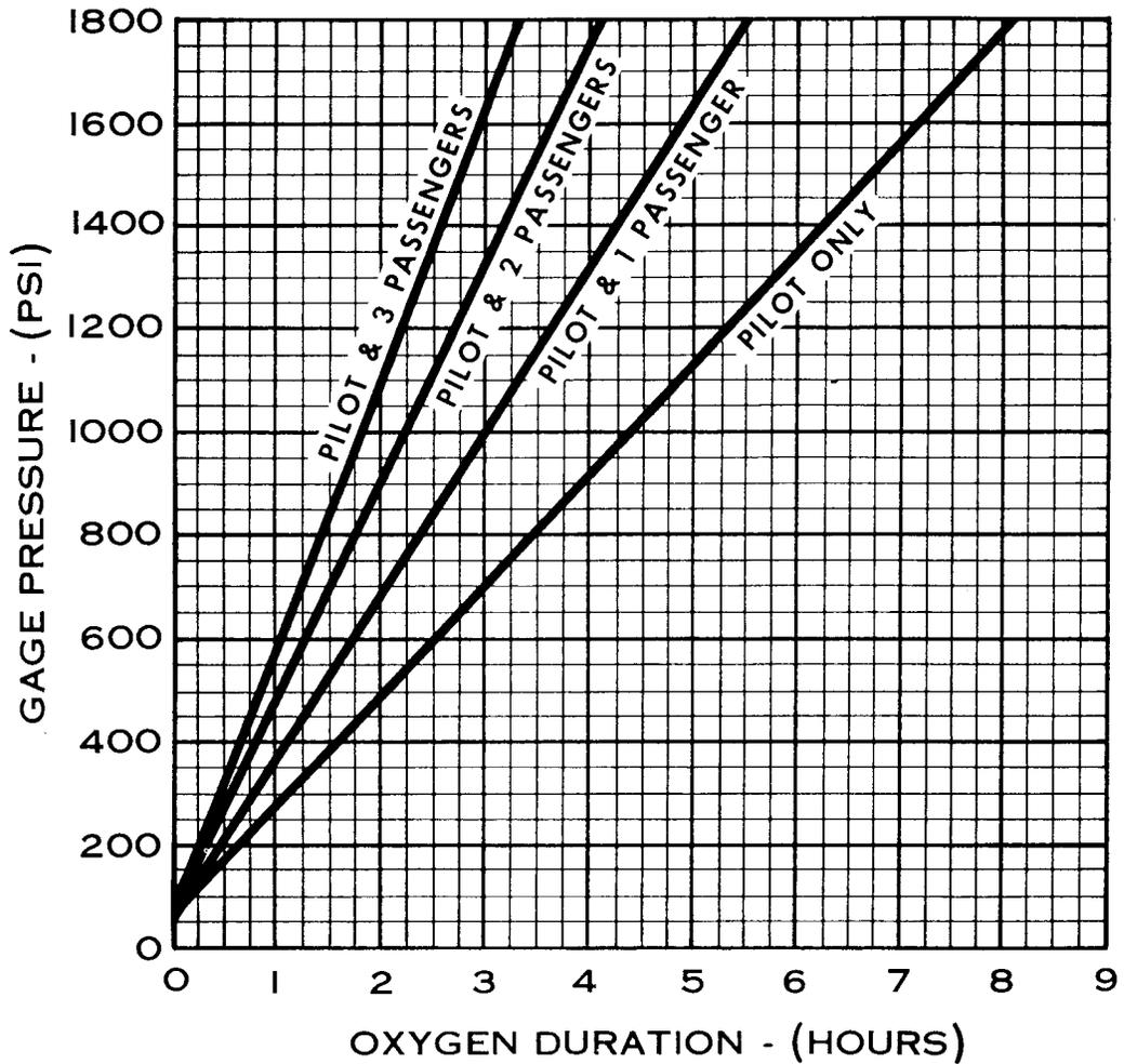
NOTE: This chart is based on a pilot with an orange color-coded oxygen line fitting and passengers with green color-coded line fittings.
