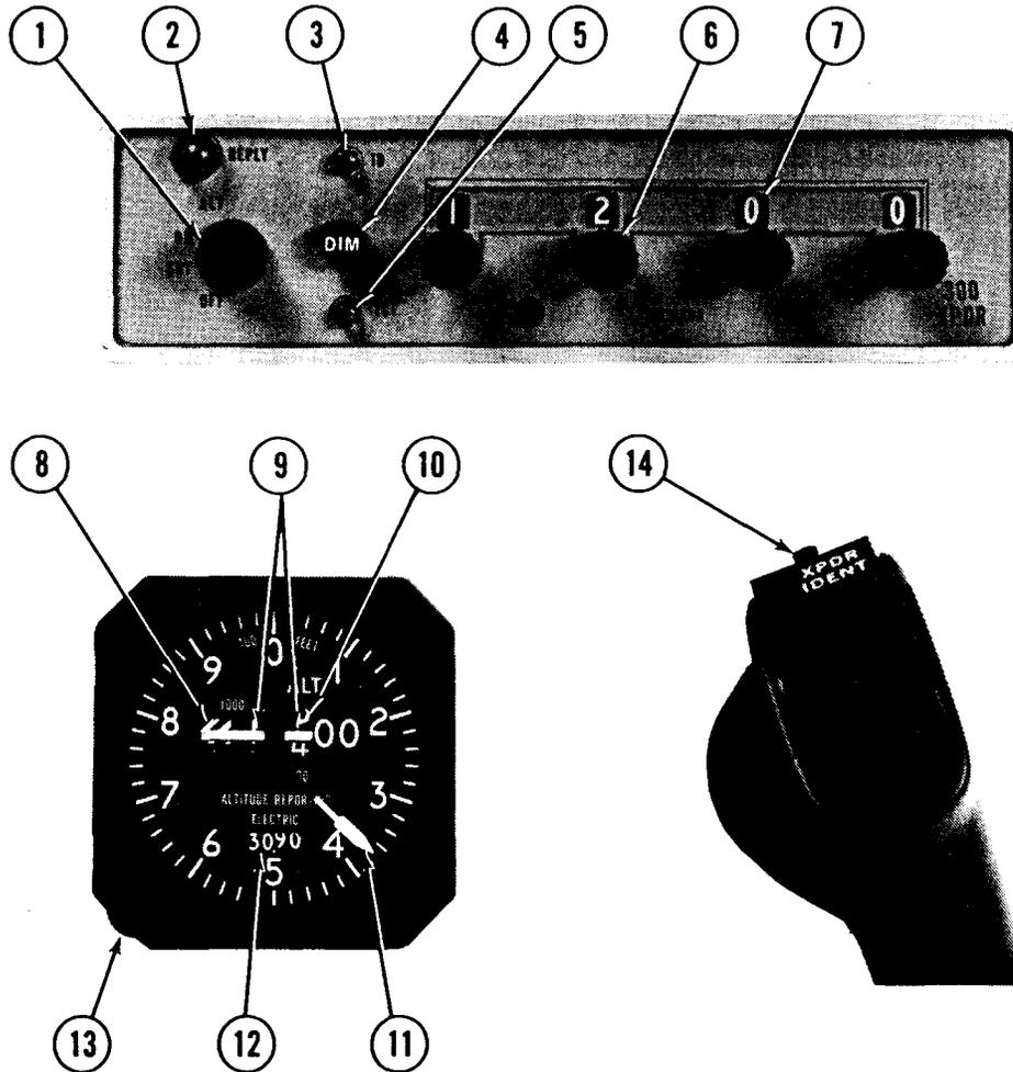
1. FUNCTION SWITCH - Controls application of power and selects transponder operating mode as follows:
