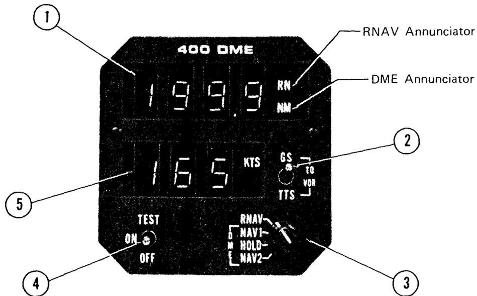
1. DISTANCE DISPLAY - In NAV 1, NAV 2, or HOLD mode, displays distance to selected VOR/DME station in nautical miles; only NM (Nautical Miles) annunciator lights. In RNAV mode, displays distance to selected waypoint in nautical miles; both RN (RNAV) and NM annunciators light.
