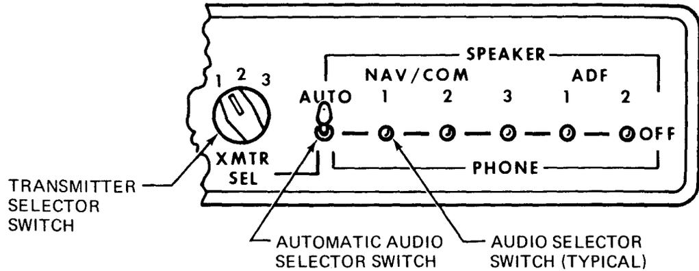
As illustrated, the number 1 transmitter is selected, the AUTO selector switch is in the SPEAKER position, and the NAV/COM 1, 2 and 3 and ADF 1 and 2 audio selector switches are in the OFF position. With the switches set as shown, the pilot will transmit on the number 1 transmitter and hear the number 1 NAV/COM receiver through the airplane speaker.
