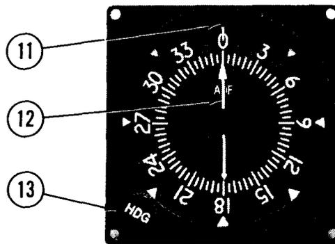
Figure 1. Cessna 400 ADF Operating Controls and Indicator
