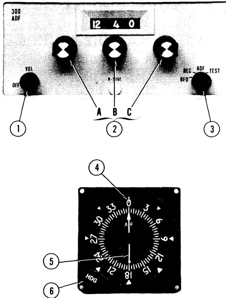
1. OFF/VOL CONTROL - Controls primary power and audio output level. Clockwise rotation from OFF position applies primary power to receiver; further clockwise rotation increases audio level.
