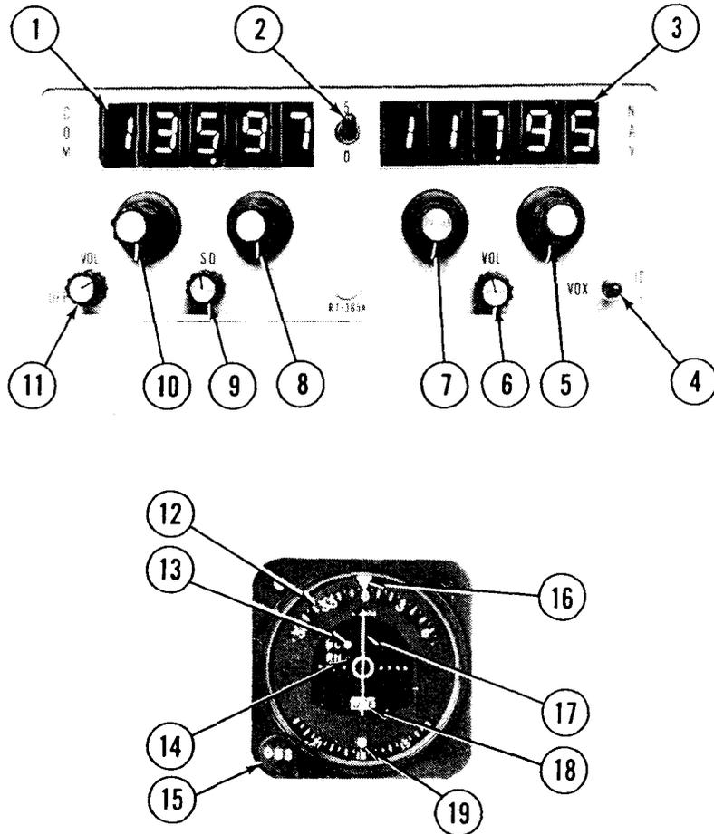
1. COMMUNICATION OPERATING FREQUENCY READOUT (Third-decimal-place is shown by the position of the "5-0" switch).
