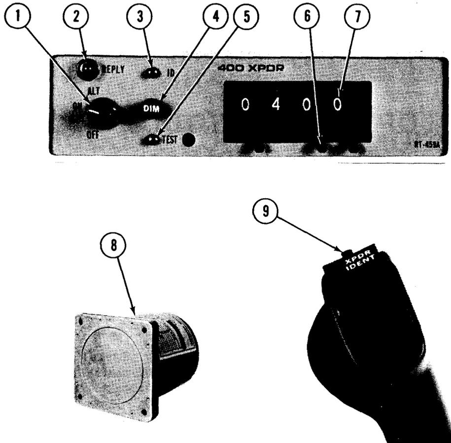
1. **FUNCTION SWITCH** - Controls application of power and selects transponder operating mode as follows:
