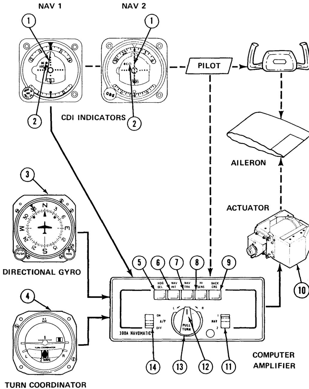
Figure 1. Cessna 300A Autopilot, Operating Controls and Indicators
