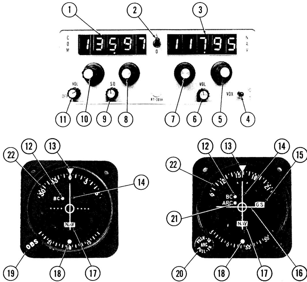
1. COMMUNICATION OPERATING FREQUENCY READOUT (Third-decimal-place is shown by the position of the "5-0" switch).
