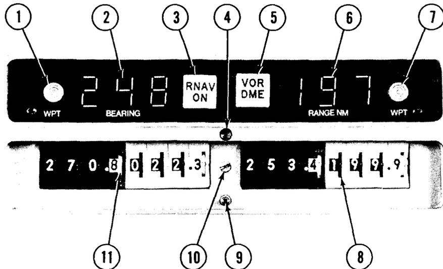
1. WAYPOINT PUSHBUTTON (WPT) - Activates the waypoint data dialed into the left side thumbwheels (11). When pressed, the WPT pushbutton lights to indicate which waypoint is "active". The WPT pushbutton light intensity is controlled by a photocell (4).
