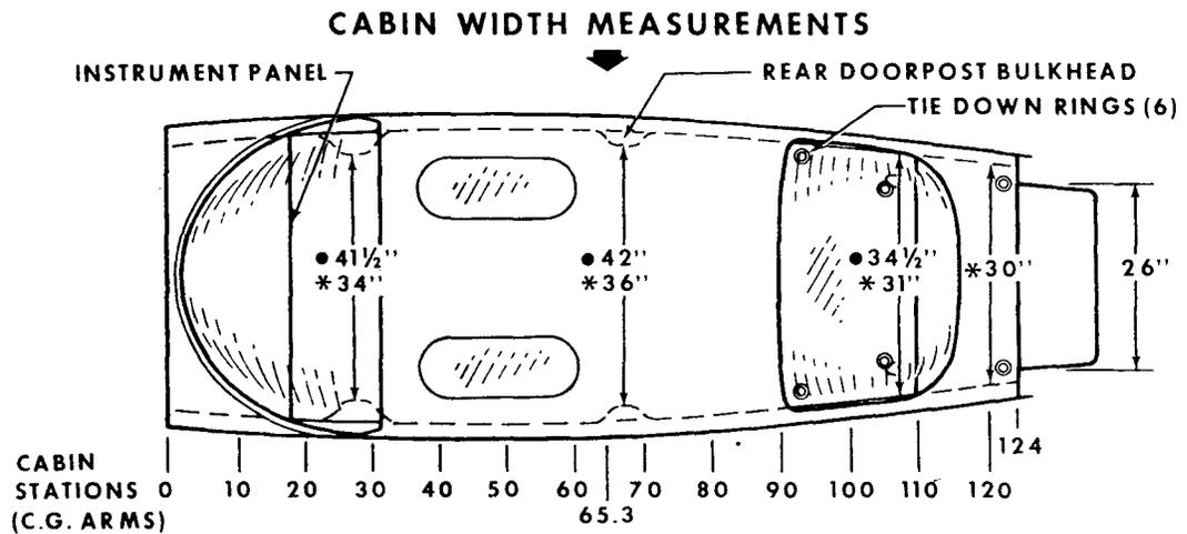
Figure 6-4. Internal Cabin Dimensions
