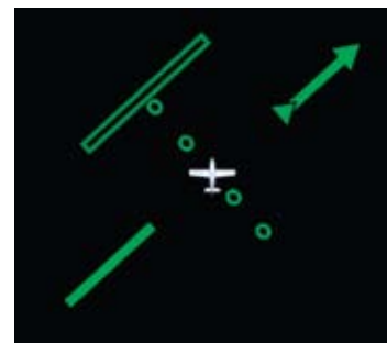
Figure 3-26 CDI Shown Hollow at Full-Scale Deflection
