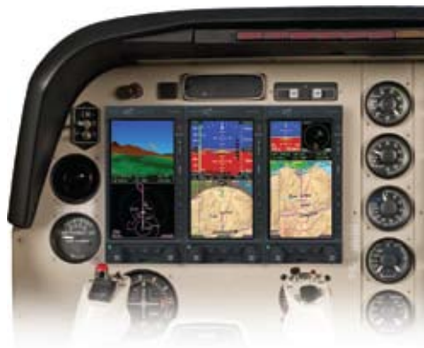
Figure 1-4 Three-tube system: PFD & dual MFDs
