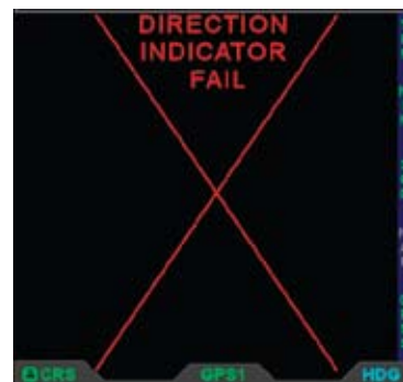
Figure 4-79 Direction Indicator Fail
