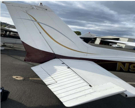
Figure 1 - Horizontal stabilizer with elevator and trim tab
