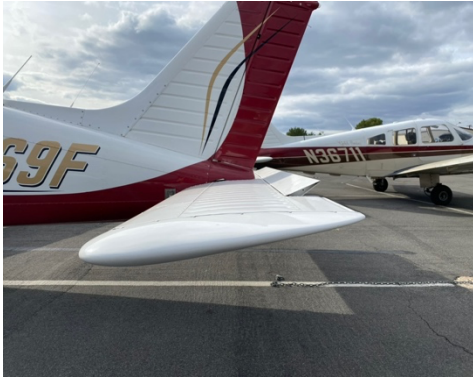
Figure 3 – Anti-servo tab and stabilator (servo) in the upward direction.
