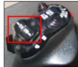
Electric Trim Switch
