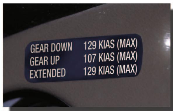
Figure 11-11. Placarded gear speeds in the cockpit.
