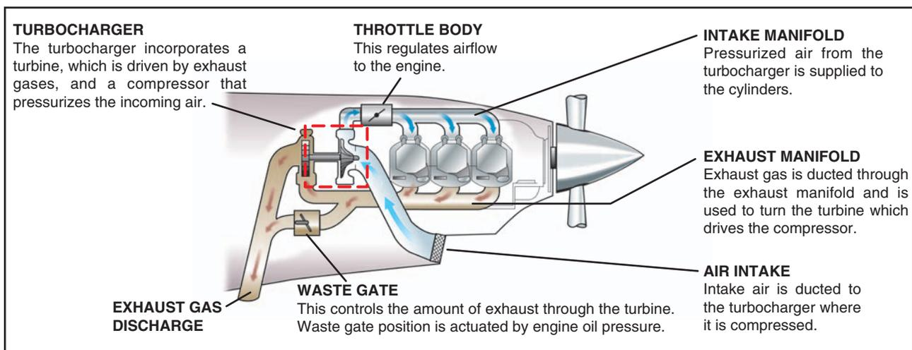
Figure 11-5. Turbocharging system.
