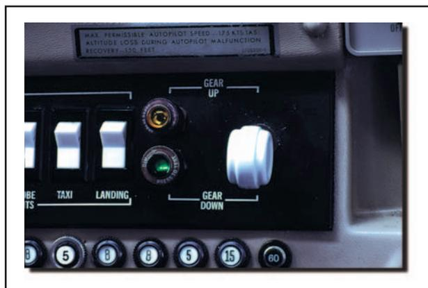
Figure 11-7. Typical landing gear switches and position indicators.
