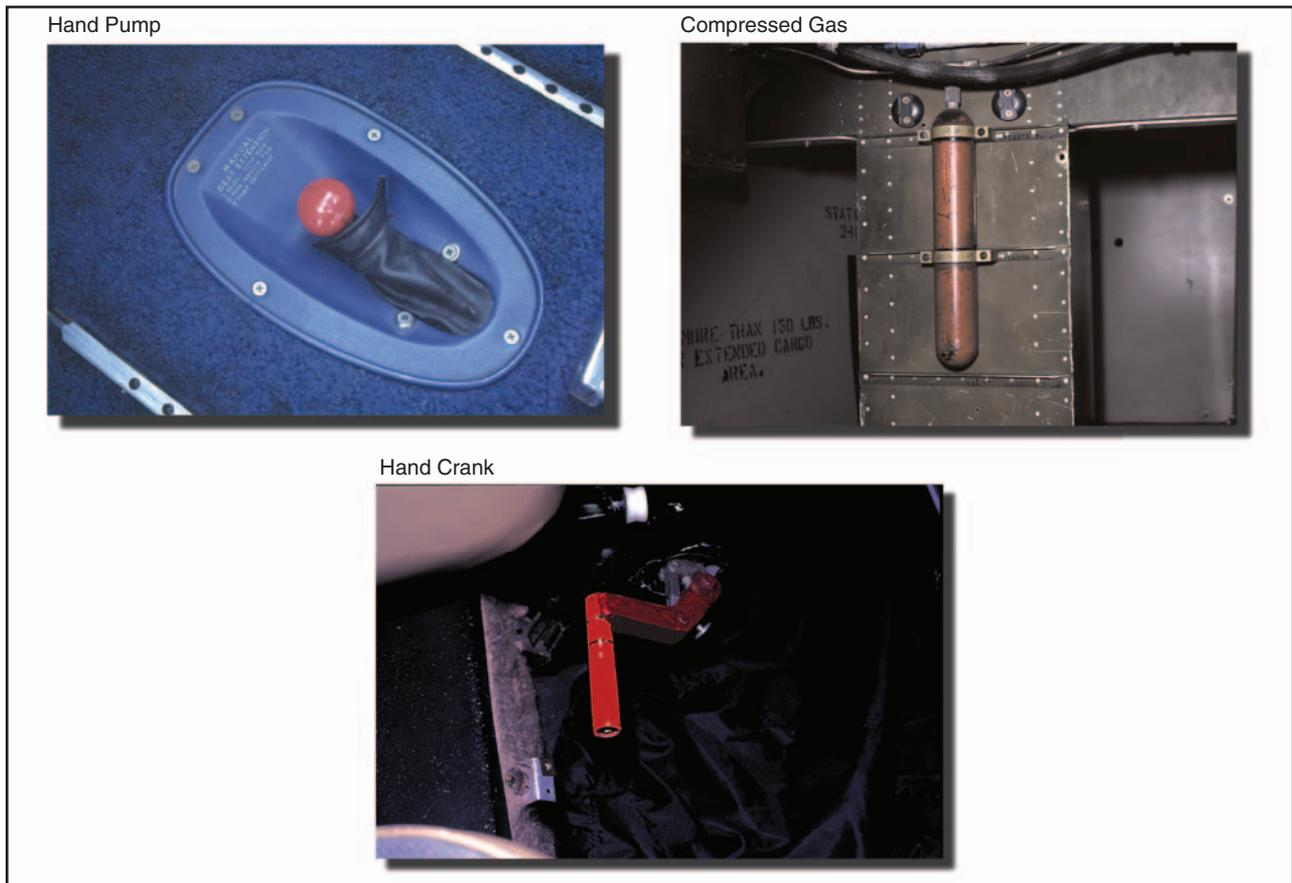
Figure 11-9. Typical emergency gear extension systems.
