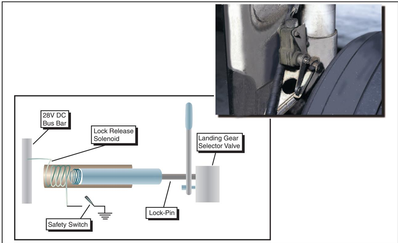
Figure 11-8. Landing gear safety switch.
