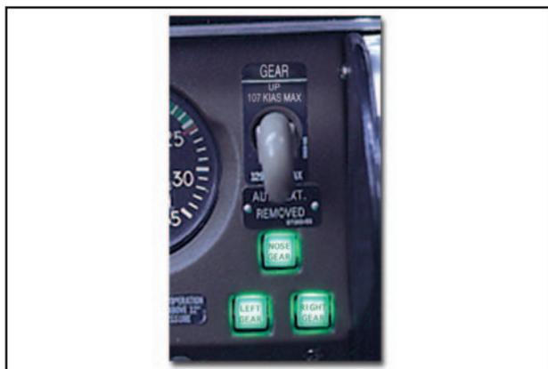
Figure 11-6. Typical landing gear switches and position indicators.
