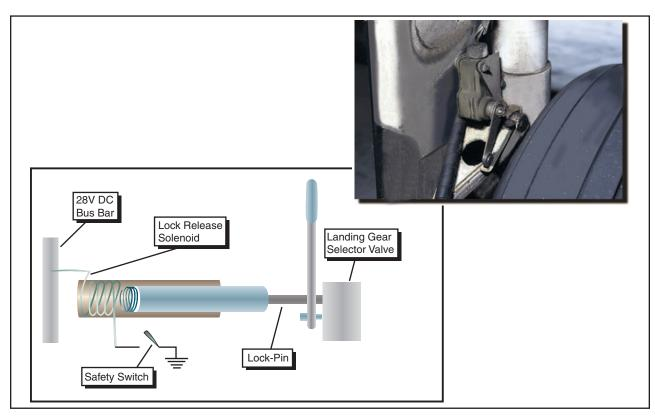
Figure 11-8. Landing gear safety switch.
