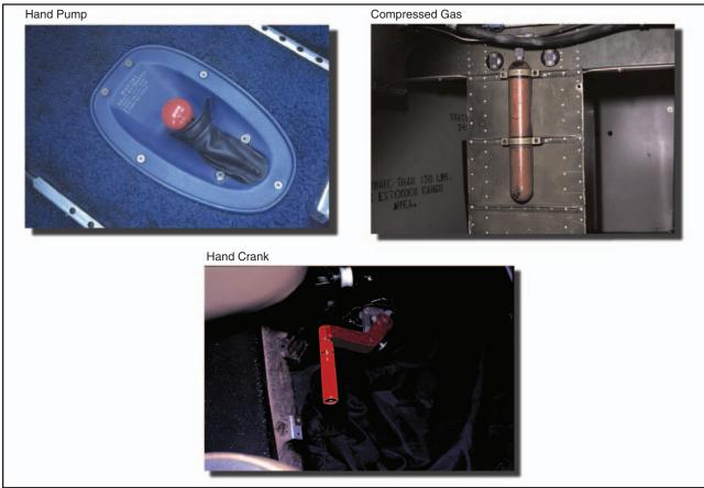
Figure 11-9. Typical emergency gear extension systems.
