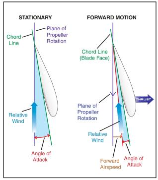
Figure 11-3. Propeller blade angle.
