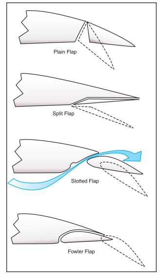
Figure 11-2. Four basic types of flaps.
