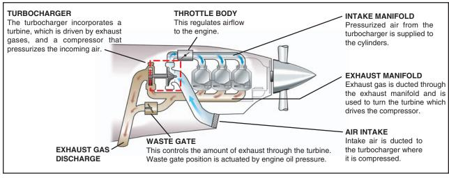
Figure 11-5. Turbocharging system.
