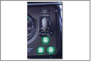
Figure 11-6. Typical landing gear switches and position indicators.
