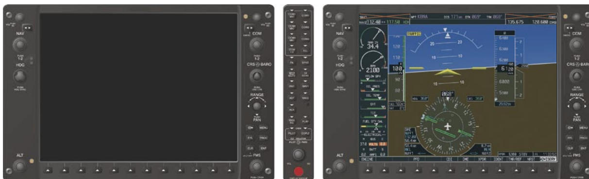
Figure 1-7 Reversionary Mode (Failed PFD)
