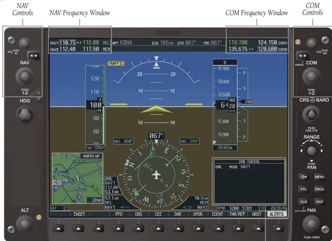
Figure 3-1 G1000 NAV/COM Interface (PFD)
