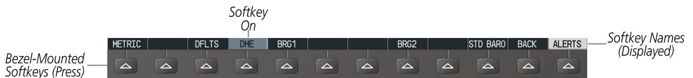
Figure 1-14 Softkeys (Second-Level PFD Configuration)
