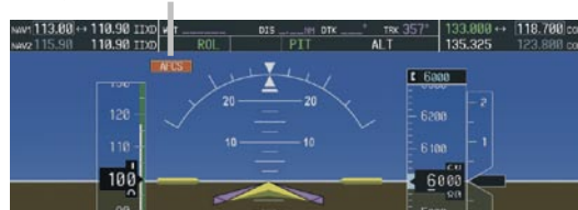
Figure A-6 AFCS System Status Field
