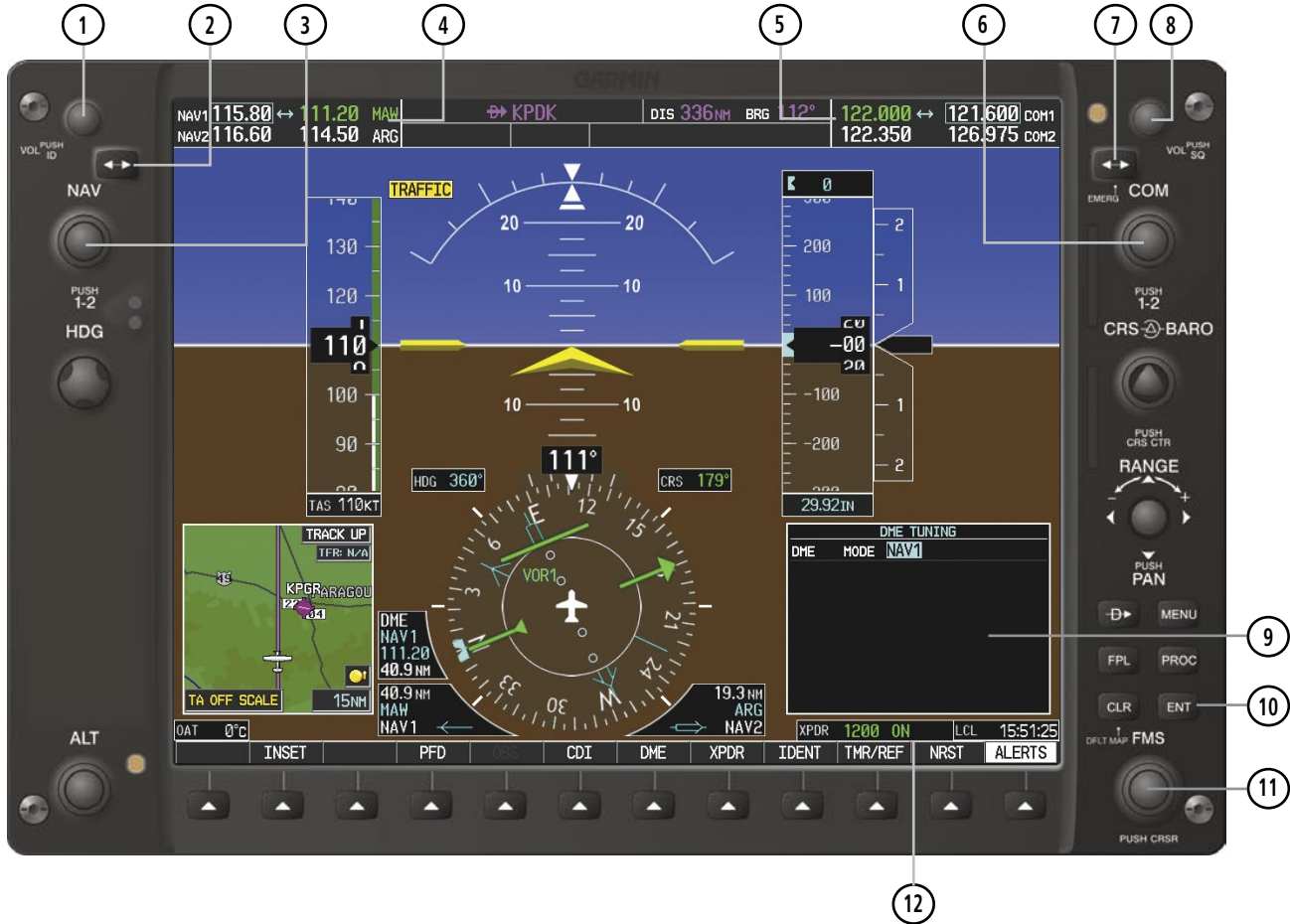
Figure 4-1 PFD/MFD Controls, COM/NAV Frequency Tuning Boxes, and DME Tuning Window (Cessna 172 PFD Shown)
