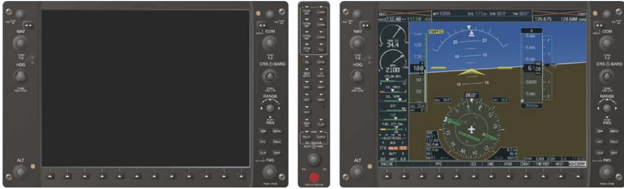
Figure 1-9 Reversionary Mode (Failed PFD)
