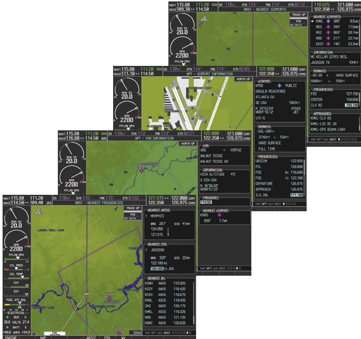
Figure 4-28 NRST – Nearest Frequencies, WPT – VOR Information, WPT – Airport Information, and NRST – Nearest Airports Pages
