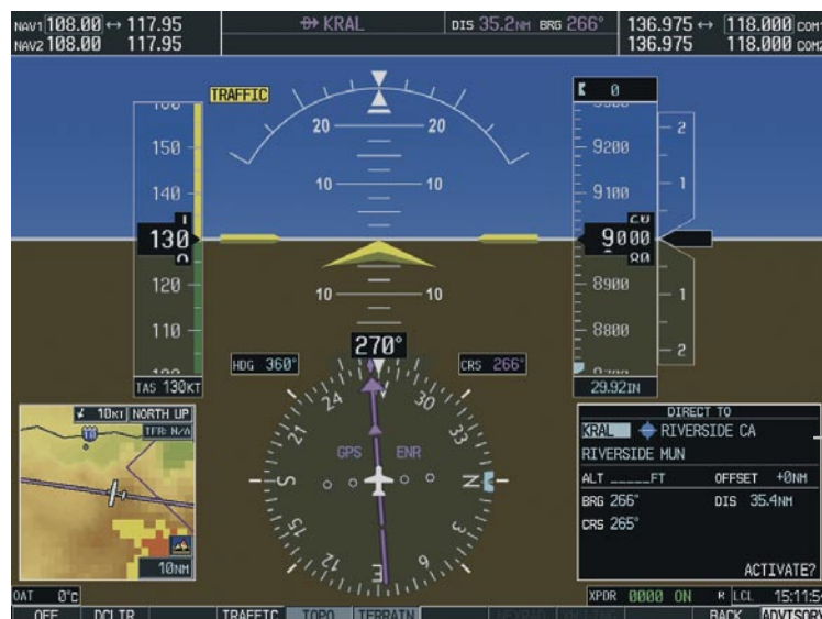
Figure 5-21 PFD Window Location
