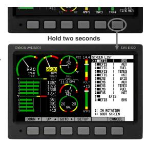
With no menus displayed, pressing button six for two seconds displays the SCREEN LIST menu, from which you may switch to, and set up, various screen configurations.
