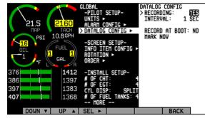
log retrieved by your PC, allowing you to quickly find the place in your data when you marked the record. For information about retrieving data and reading the file produced, please see the help file included in the Dynon Product Support Program (version 3.0 and higher). Note that the internal data log only includes data for the engine monitor portion of the EMS-D120. EFIS data is not logged.
