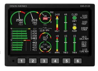
User interaction takes place via the EMS-D120 main display and the six buttons beneath. Note: buttons are not labeled on actual product
