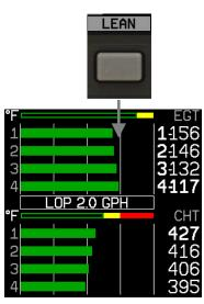
In the above example, cylinder 1's EGT peaked first and cylinder 4's EGT peaked last. There was a total decrease of 2.0 GPH in fuel flow between the first and last cylinder peak, indicating lean-of-peak
